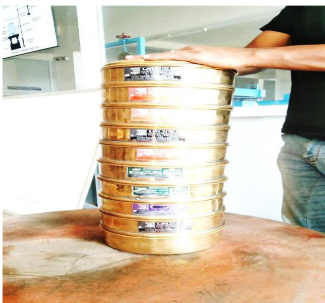
Fig.5. IS set of sieves
